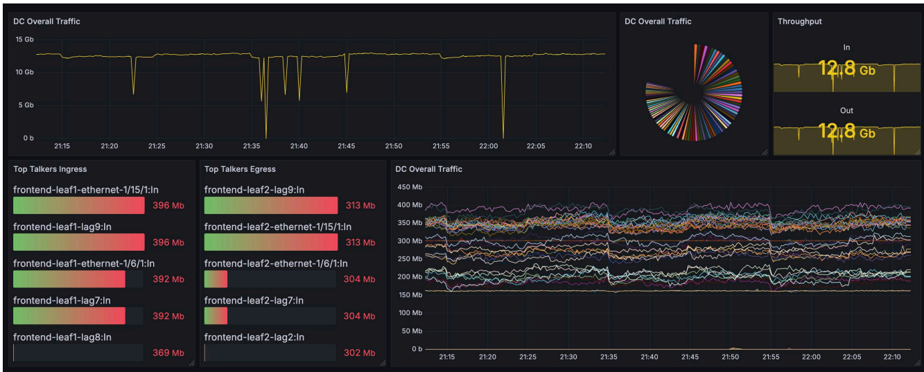
View 1: This dashboard shows statistics collectively from all the data center nodes. At the top right, the display shows the total traffic trend, below that the Top Talkers interfaces in both directions, and to the left, individual nodes with their traffic trend.
